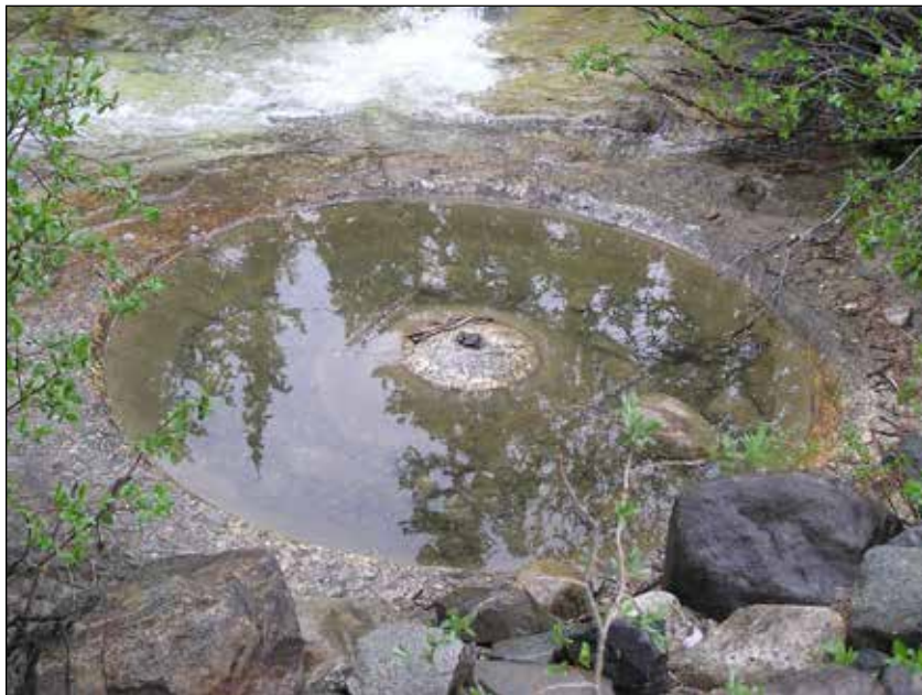
Numerous burro-powered arrastras once existed in South Park, crushing ore into gravel to release valuable minerals. Photo courtesy Linda Balough.
